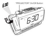
3. If the image appears to be upside down on your wall or ceiling when you are lying in bed, set the **FLIP IMAGE switch** to its alternate position.
